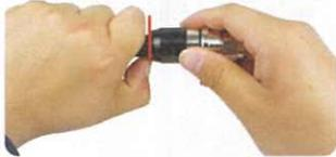
Push and twist the connector onto cable until it reaches the cable mark. The installer will hear two "clicks" during this process.
