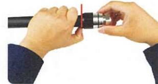
Push and twist the connector onto cable until it reaches the cable mark. The installer will hear two "clicks" during this process.
