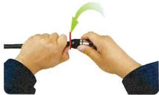
**Twist the connector clockwise onto cable** until it does not rotate or reaches the cable mark.
