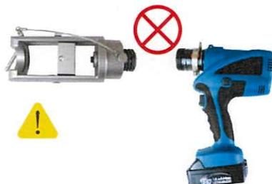
If it is not necessary, do not disassemble it at will, so as not to cause oil gun leakage.
